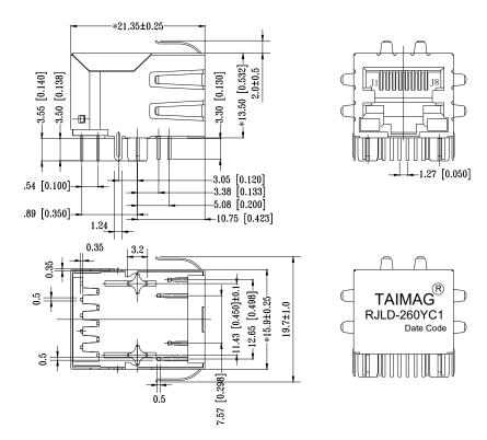
PCB Layout: mm;TOLERANCE:±0.10
