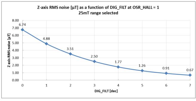
Figure 19: Z axis RMS noise (typ) without temperature compensation and 25mT range selected
