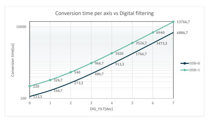
Figure 5: Conversion time vs. digital filtering (DIG\_FILT) at typical Fclk = 2.4MHz
