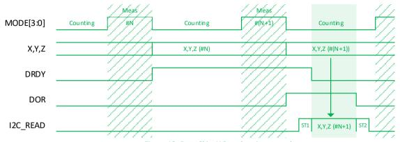
Figure 12: Data Skip: When data is not read
