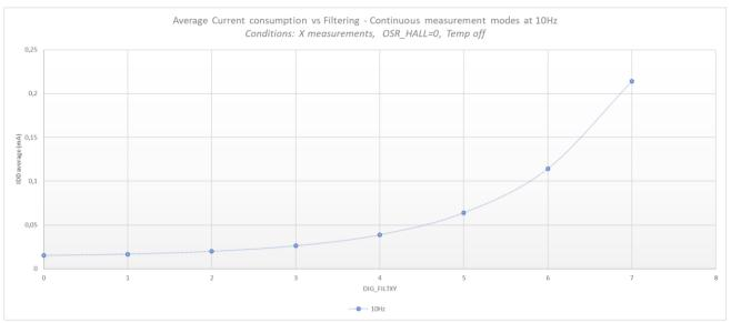
Figure 4: Average consumption vs Filtering – Continuous measurements at 10Hz – Temperature compensation off
