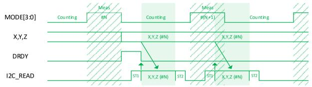
Figure 11: Data read start during measurement
