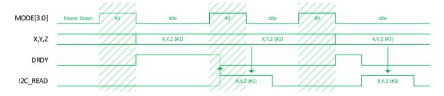
Figure 8: Single measurement mode when data read started during measurement period
