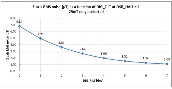
Figure 23: Z axis RMS noise (typ) with temperature compensation and 25mT range selected
