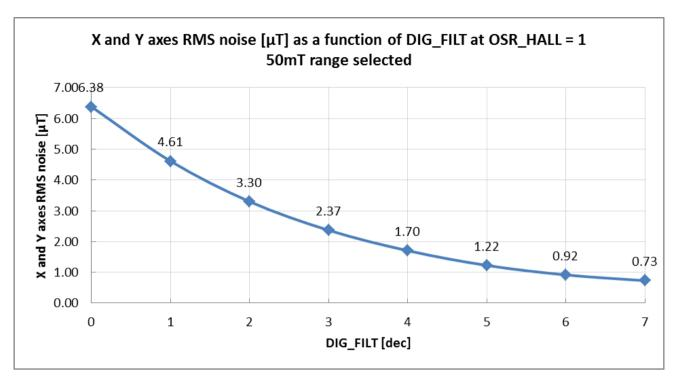
Figure 20: XY axis RMS noise (typ) without temperature compensation and 50mT range selected
