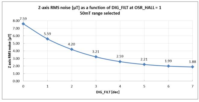
Figure 25: Z axis RMS noise (typ) with temperature compensation and 50mT range selected
