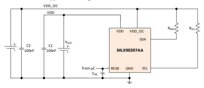
Figure 26: Recommended application diagram
