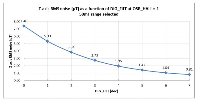
Figure 21: Z axis RMS noise (typ) without temperature compensation and 50mT range selected
